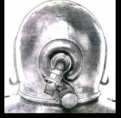
Edward's circuitous exhaust valve, with the air inlet at its centre.
